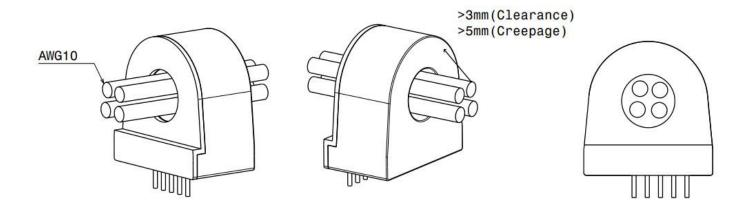
Reinforced insulation, insulation material group III, pollution degree 2, altitude < 5,000 m and overvoltage category II. Please take enough creepage distance between each pin.
